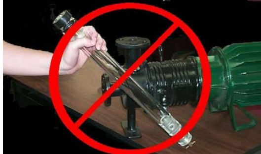
Do Not Over-Tighten the Leveler
