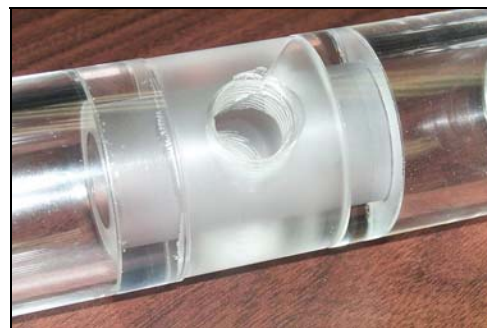
Over-Tightening can result in cracking
