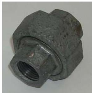
Problem solved! Proper vertical alignment is easily attained with the use of a union and there is no longer a threat of over-tightening the connection and cracking the Level Monitor.
