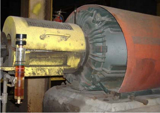
An OSGL installed on a bearing housing at Cargill Salt.
