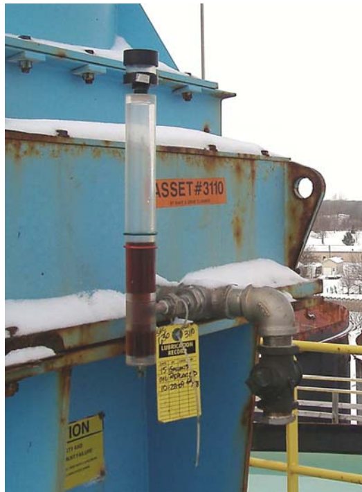
Exposure to cold weather is not a problem for the OSGL, seen here on a large gearbox.
